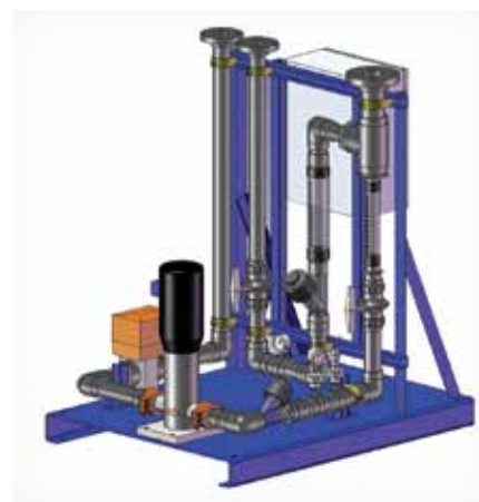
Brine Pump Skid
